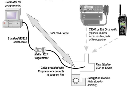
Use the cable provided with the Midian Programmer to connect the programmer to the pads on the flex circuit. See diagrams on the following pages for correct connection points.
