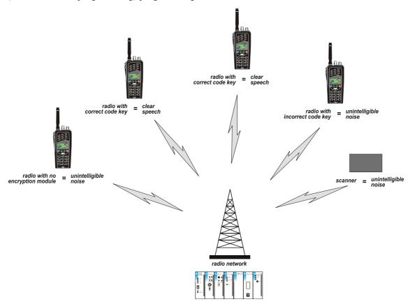
Whether or not a radio transmission is encrypted is the user's choice. When the encryption mode is selected, the radio sends and receives encrypted calls to and from other radios with compatible encryption module and settings (keys or codes). However, even when encryption is not selected, an encryption-enabled radio will always decode encrypted communication from any radio with compatible modules and settings.
