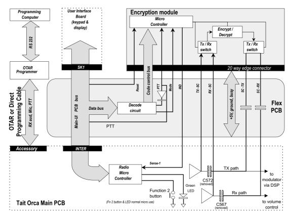
An addressable latch on the radio UI board is replicated on the encryption flex and driven by the same serial data bus. The radio micro uses four outputs of this latch to control the encryption code select bus. Two other outputs provide the PTT and Mode drives to the module. The remaining two pins function as normal for the UI board and are unused on the flex.
